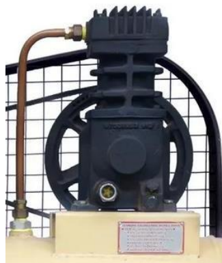
Fig. 5.6: Single Cylinder Belt Driven Air Compressor
